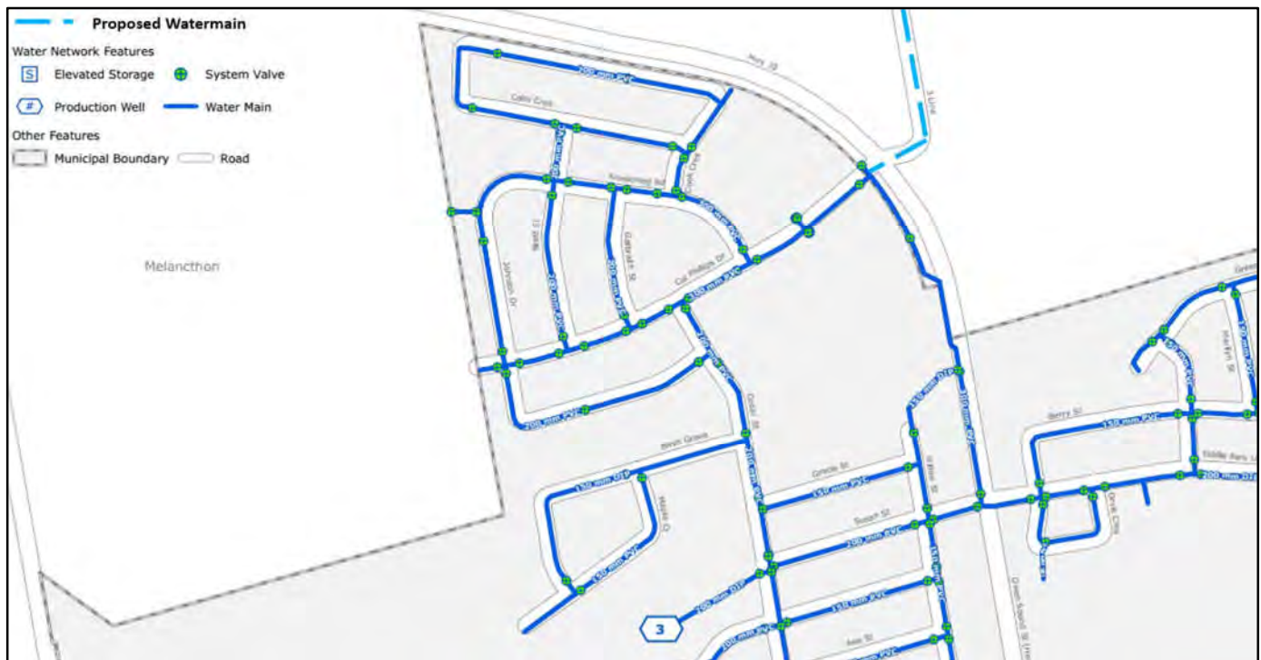
Figure 6 – Shelburne Water Distribution Network (Town of Shelburne, 2021)
