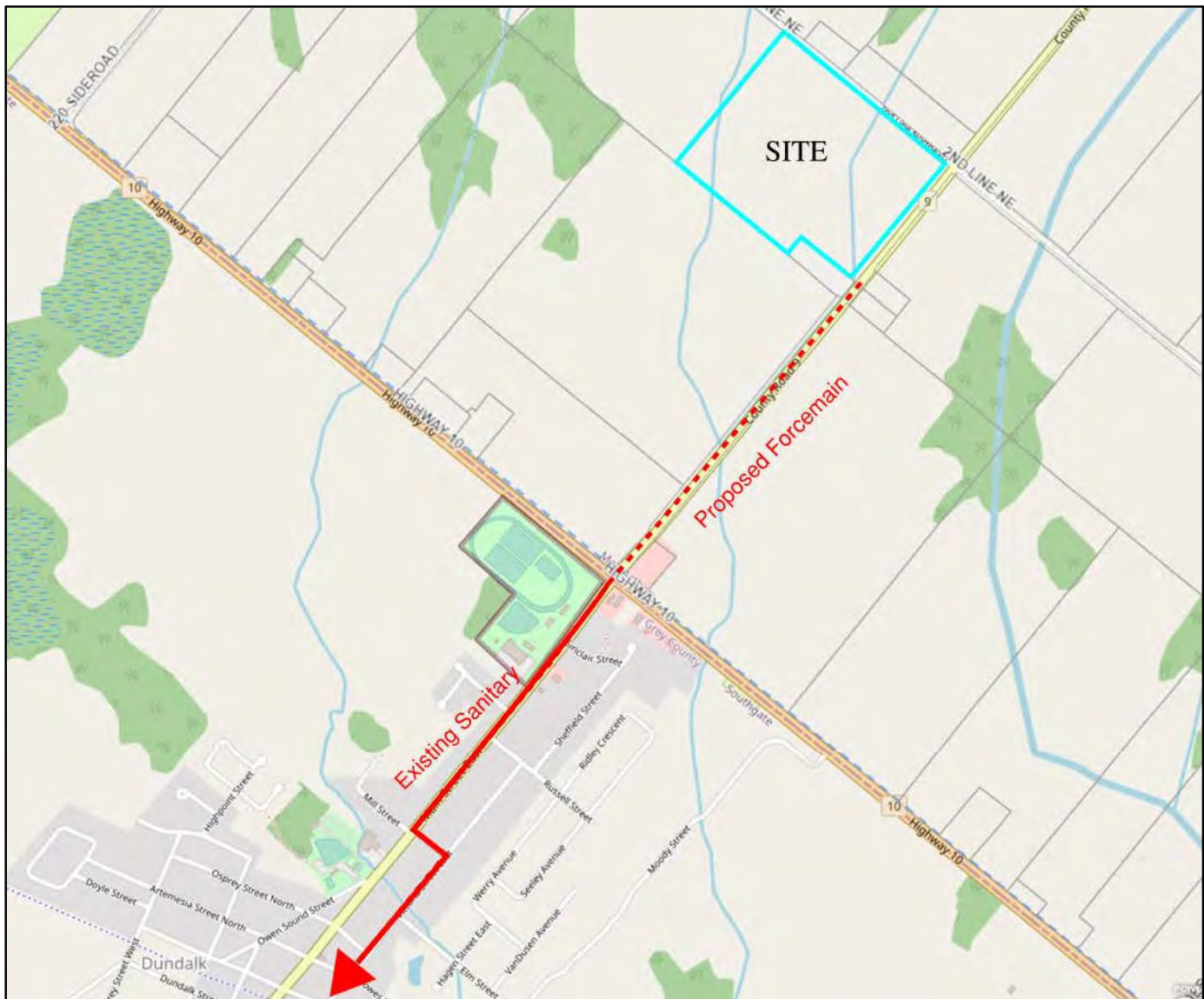
Figure 4 – Proposed Sanitary System (Dufferin County Interactive Map, 2023)
