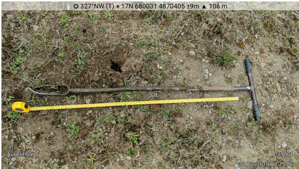
Photo 10: Likely till derived soil which has had the topsoil scraped off and placed in adjacent perimeter berm. Poor vegetative cover indicative of site disturbance and poor fertility.
