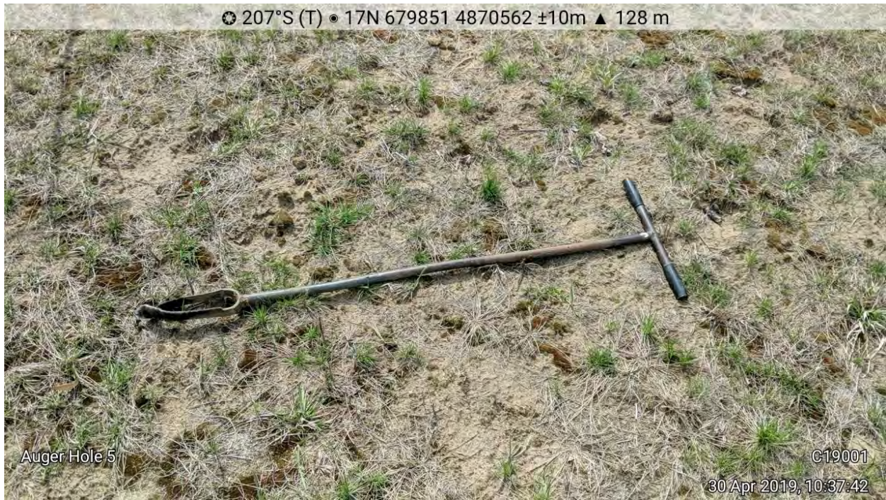
Photo 5: Rapidly drained Brighton soil – It appears that the surface (i.e., topsoil) has been removed. Soil is exposed at the surface and vegetation growth is poor.
