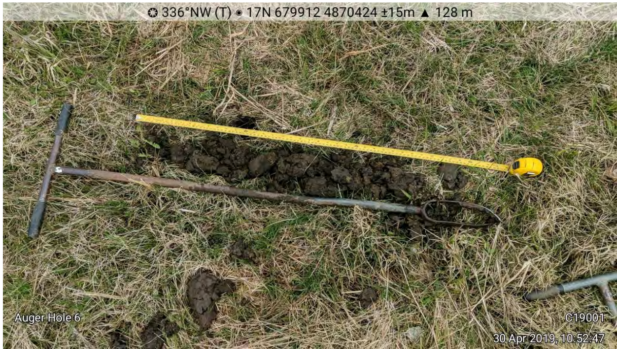
Photo 7: No soil profile development indicative of a highly disturbed site.
