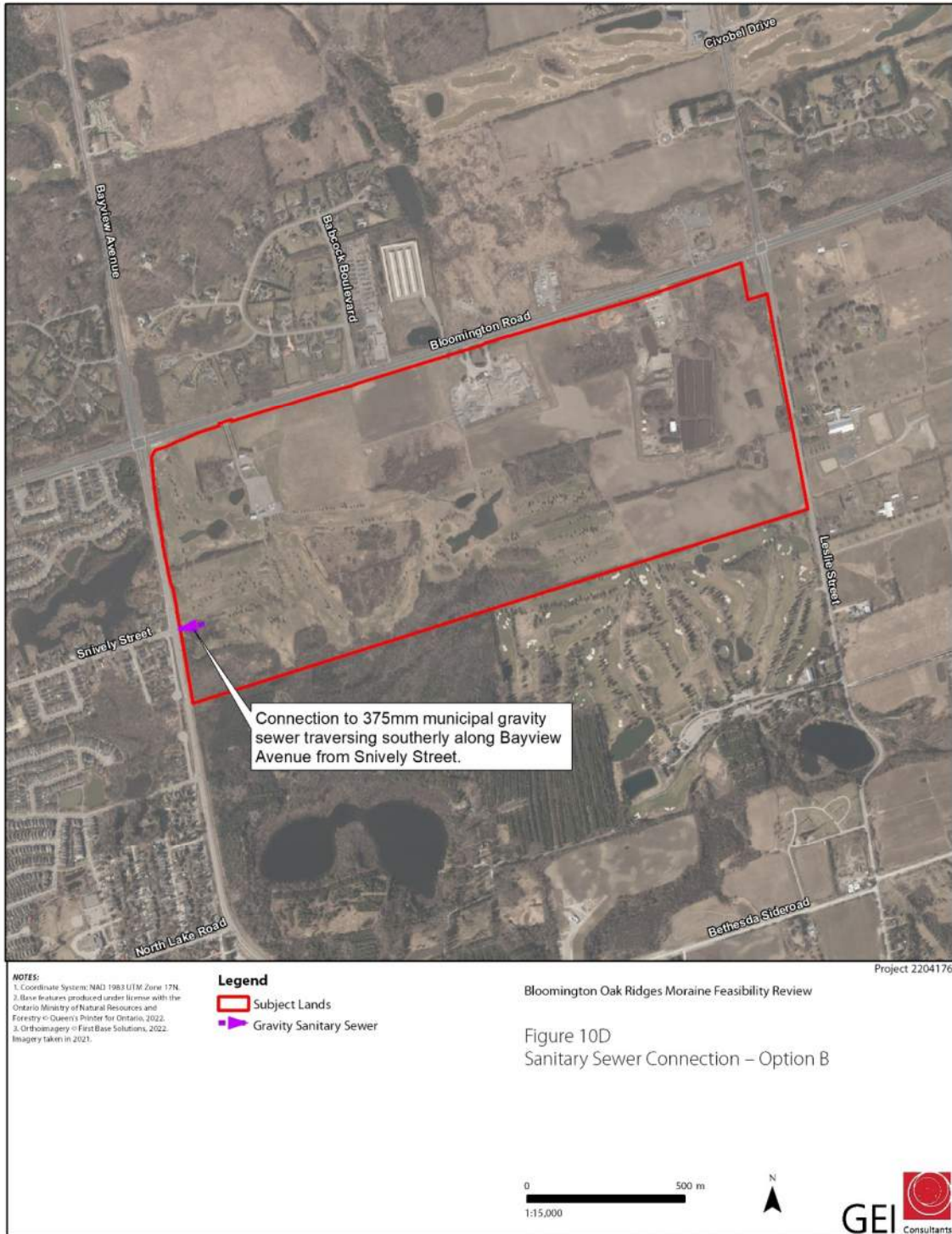
Figure 10D: Sanitary Sewer Connection – Option B
