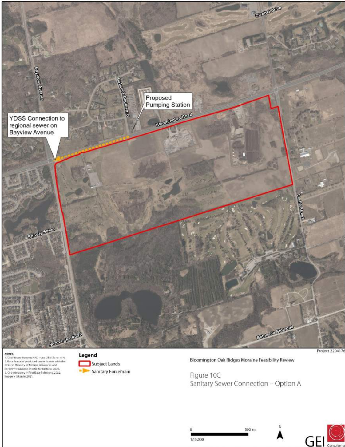
Figure 10C: Sanitary Sewer Connection – Option A
