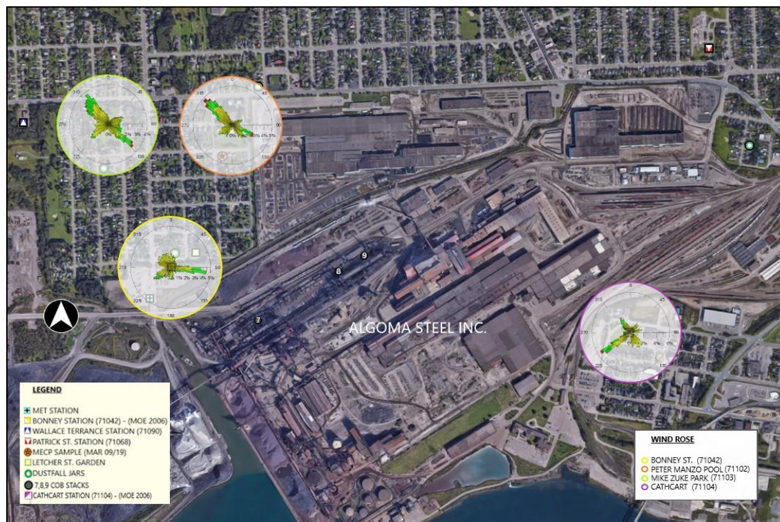
Overlay of four wind rose patterns from MOE Report, Sault Ste. Marie Particulate Monitoring Special Study (2007) page 6, figure 6 on a Modified Google Image (2020).
