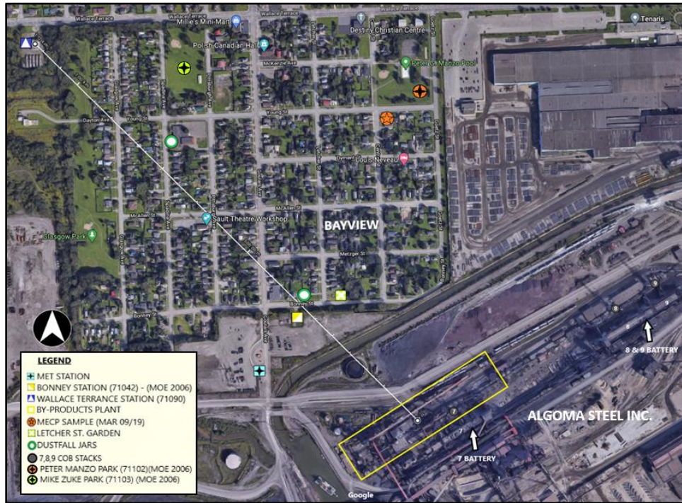
Modified google map showing monitoring devices relative to sources of benzene compounds
