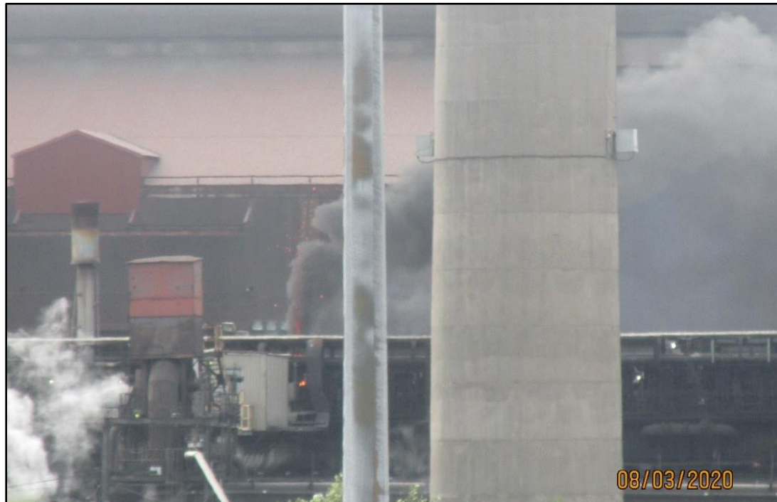
Emission resulting from soaking and the initial start of a push (removal of coke) at ASI No. 9 Battery
