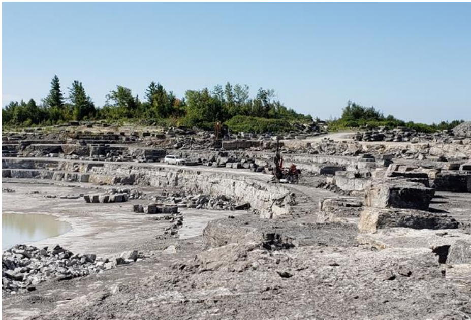
Dimension stone quarry with equipment used to mechanically remove the limestone bedrock.
