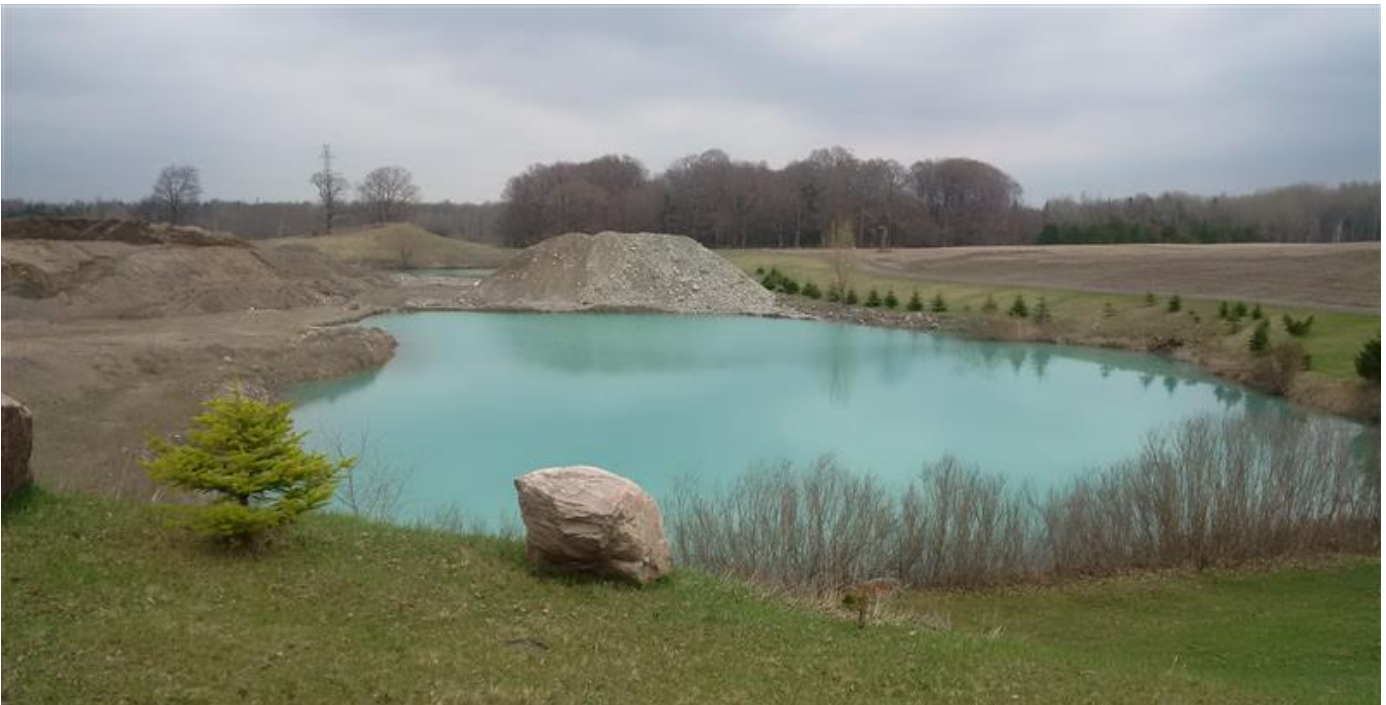
An aggregate pit where excavation has extended into the water table and one side of the pond has been rehabilitated.
