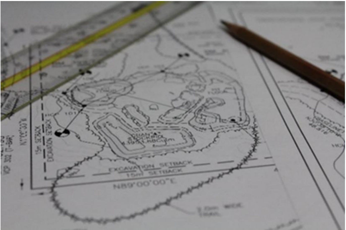
Excerpt from a site plan showing the required setback from the site boundary.
