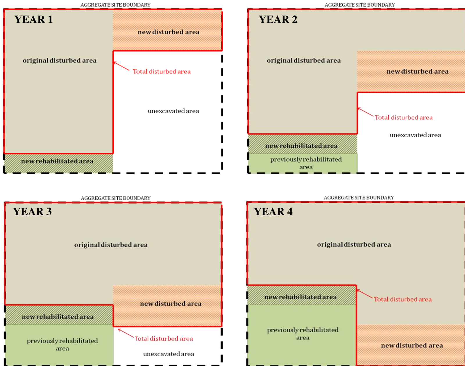
Figure 13: Example of the pattern of disturbed area versus rehabilitated area for aggregate sites in Ontario.
