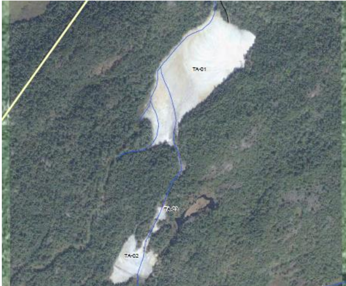
Figure 6 – Location of three tailings areas and interconnecting drainage channel (Image Source: CH2MHill 2013)
