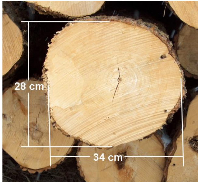
Figure 2 - Measuring diameters: logs with irregular sawn surfaces
