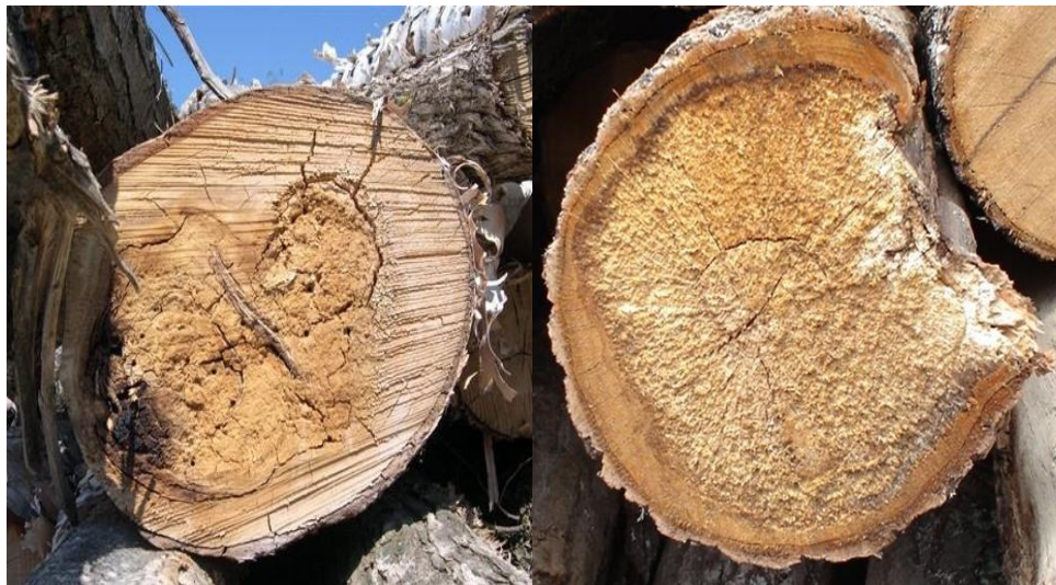
Figure 9 - Examples of punk rot
