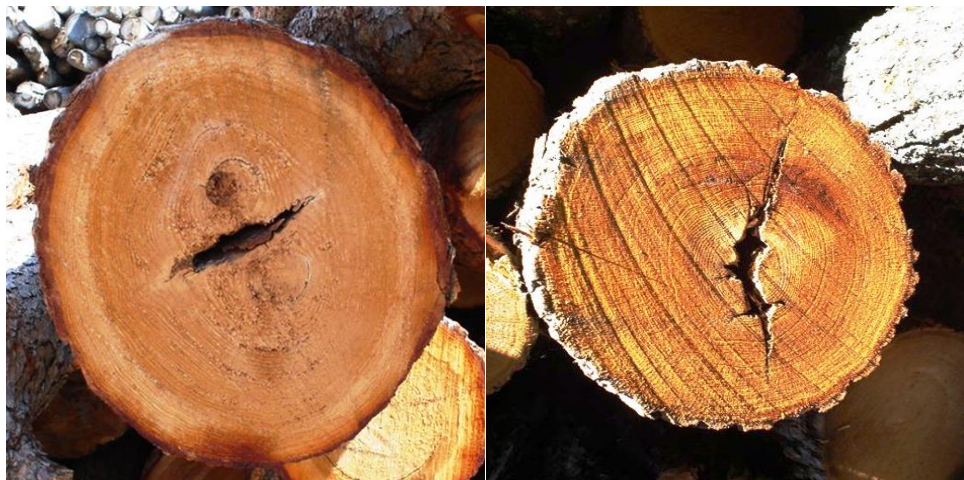
Figure 7 - Examples of heart check on the end surface of a log
