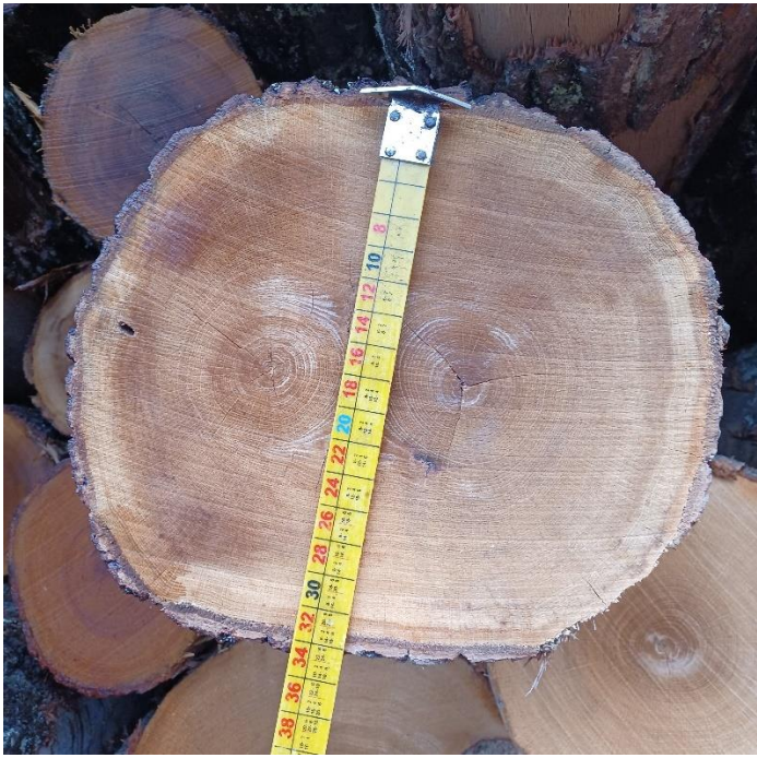
Figure 3 - Measuring diameters when cat's eyes are encountered
