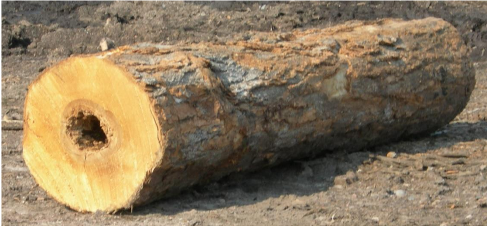
Figure 32 - A grade 1 maple log containing a partial defect
