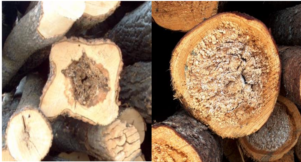
Figure 6 - Examples of stump rot
