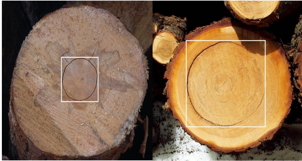
Figure 8 - Examples of shake
