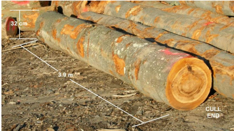
Figure 34 - A grade 2 beech log containing a defect
