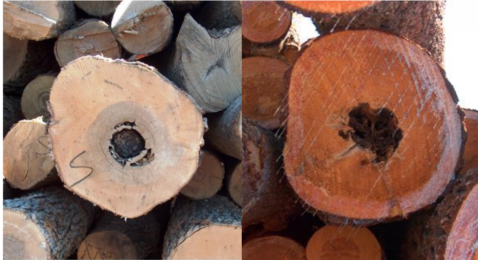
Figure 5 - Examples of heart rot
