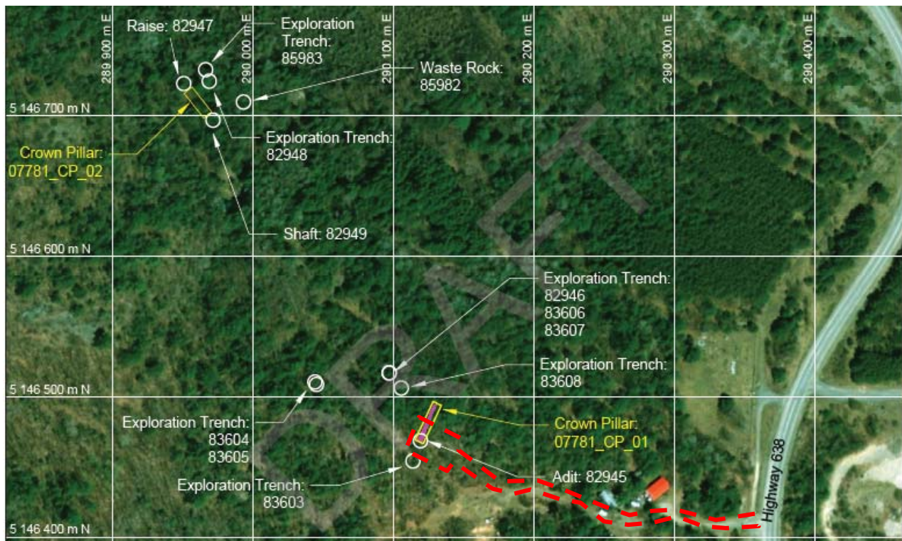
Figure 2- Location of mine hazards at the Rock Lake Mine property. The proposed rehabilitation activities will address the adit (feature ID 82945) located in Rock Lake Mine South. The boundary of the project area is defined by the site access road and area east of the adit.
