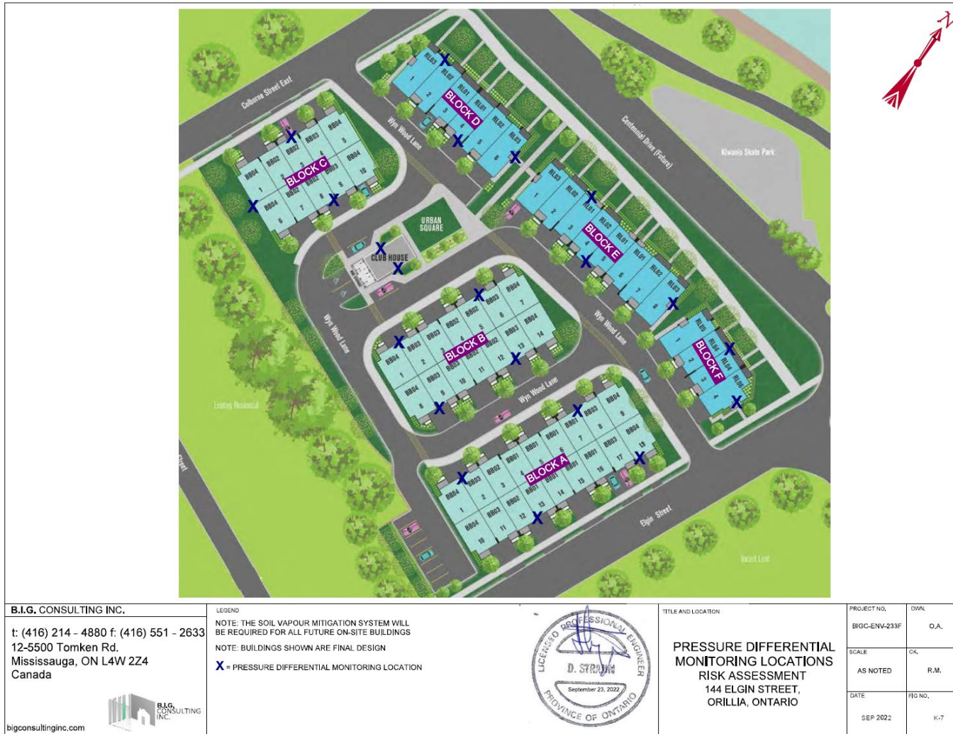
Figure K-7 “Pressure Differential Monitoring Locations, Risk Assessment, 144 Elgin Street, Orillia, Ontario” by BIG dated September 2022
