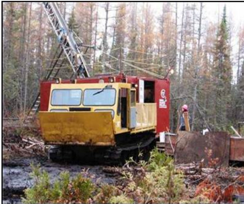
Photo 8: Diamond drill and associated equipment, greater than 150 kilograms in weight.
