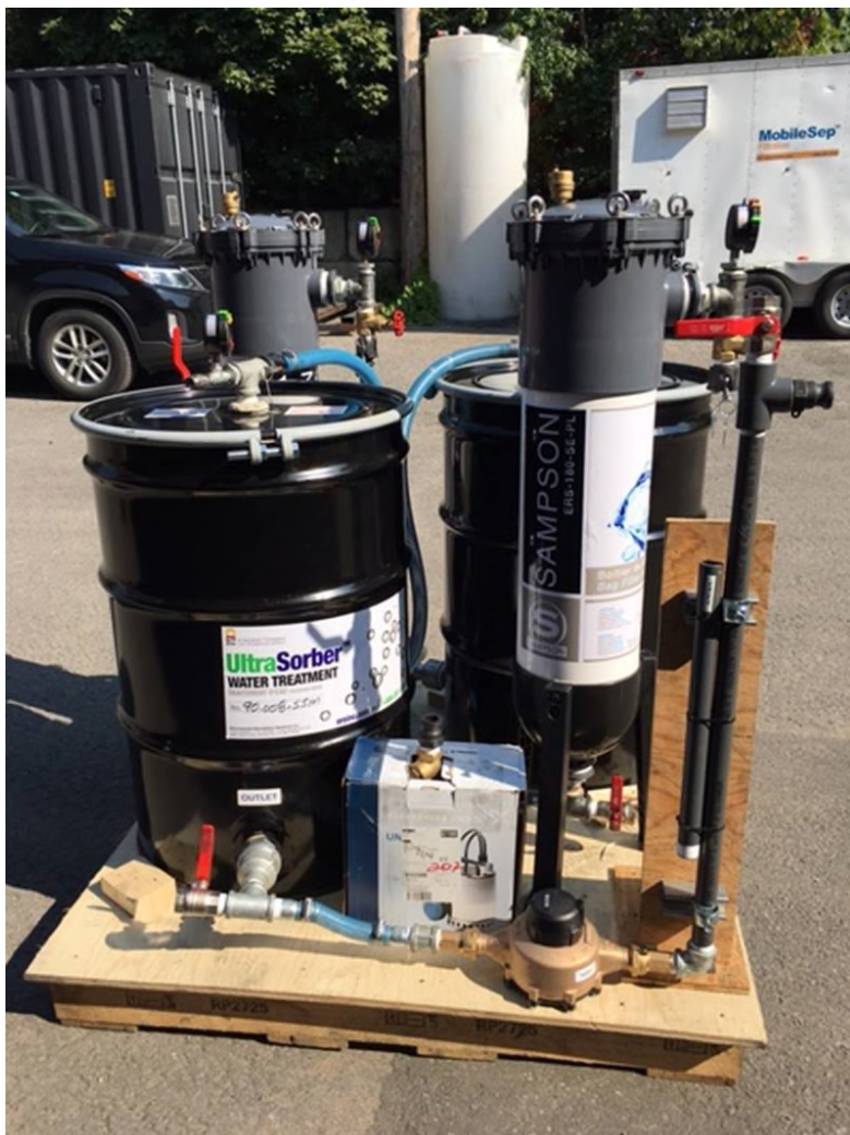
Figure 1 Typical Adsorptive Media Filtration System (source: ERE Inc.)
