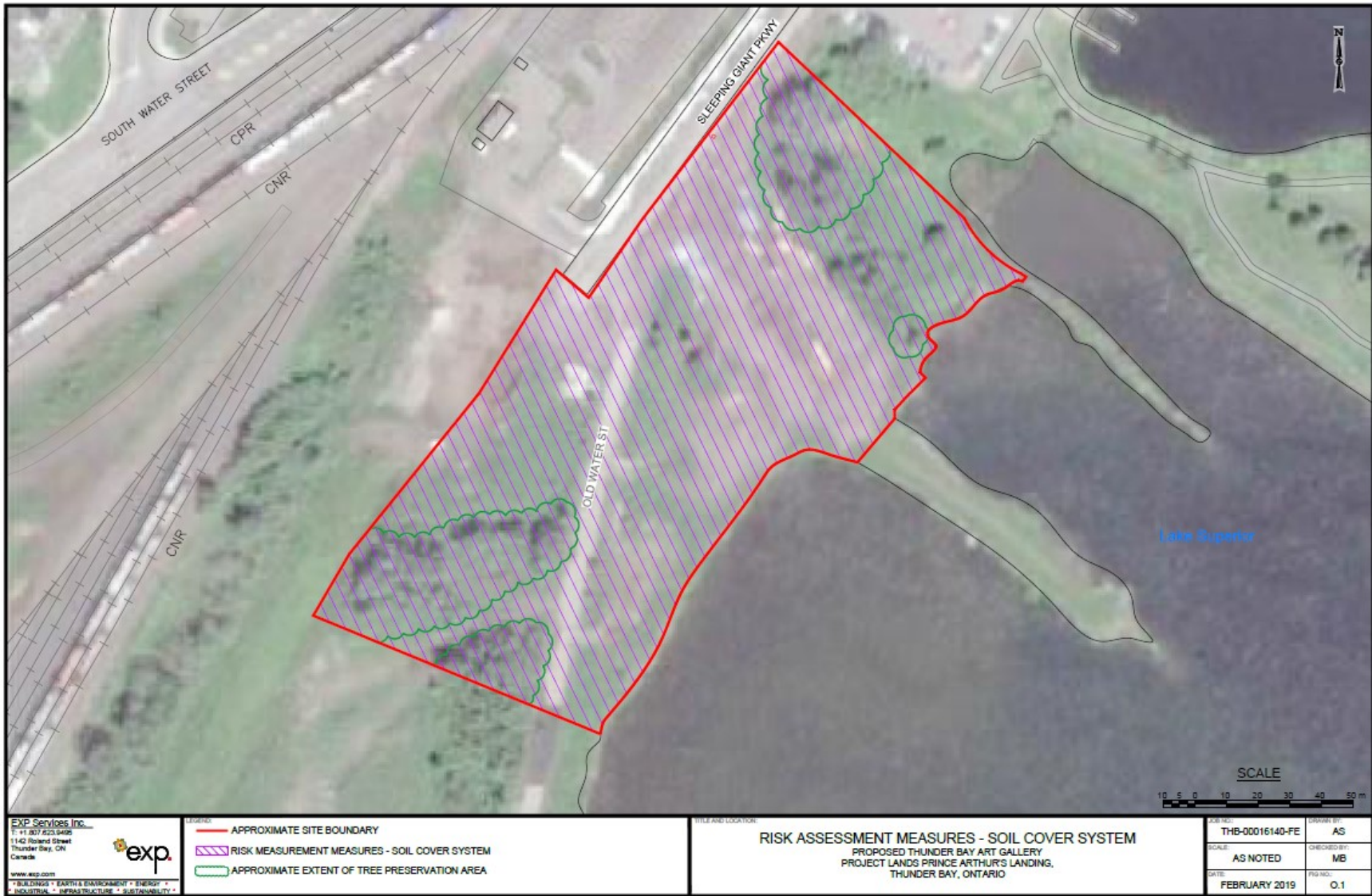
Figure O.1: "Risk Assessment Measures – Soil Cover System" by EXP, dated February 2019
