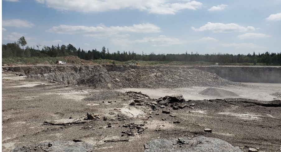
Construction aggregate limestone quarry with muck pile produced from blast.
