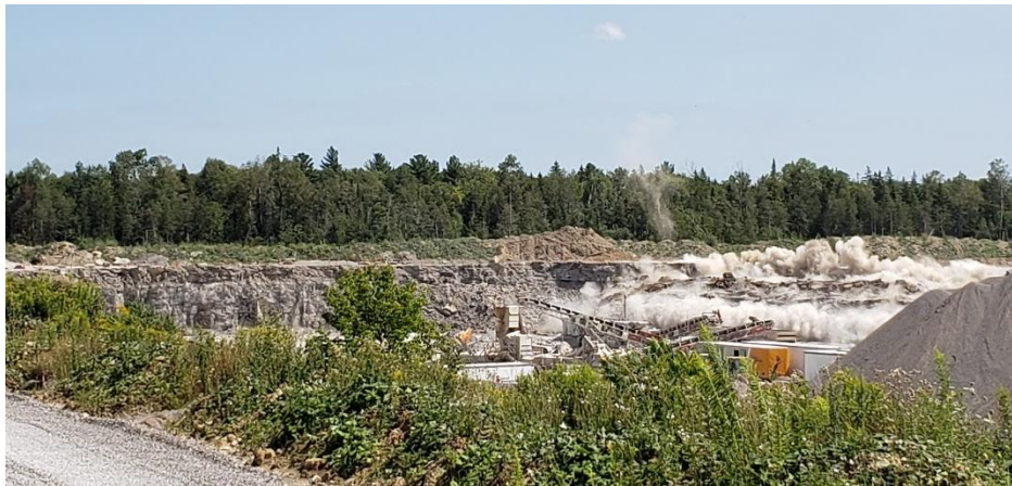
A construction aggregate limestone quarry conducting a blast.
