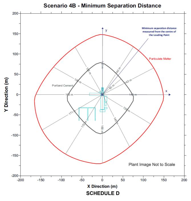
Minimum Required Separation Distances from the *Plant* to the *Points of Reception*
